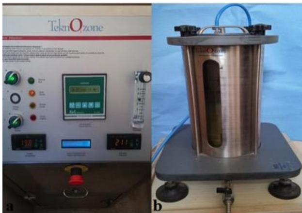
Figure 2a. Digital indicator on the generator; 2b. Reaktor tank of generator
